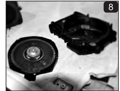
In case of the factory subwoofer is glued, be careful not to damage the plastic enclosure which can be re used for the CDT BM8-Sub1.
